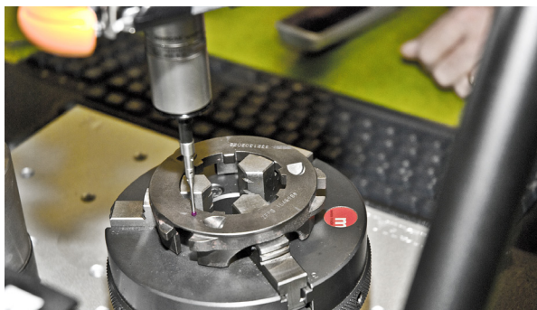
Equator measuring a ZF Marine part
