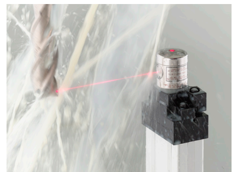
Figure 8 - Checking broken tools with the coolant system still active
