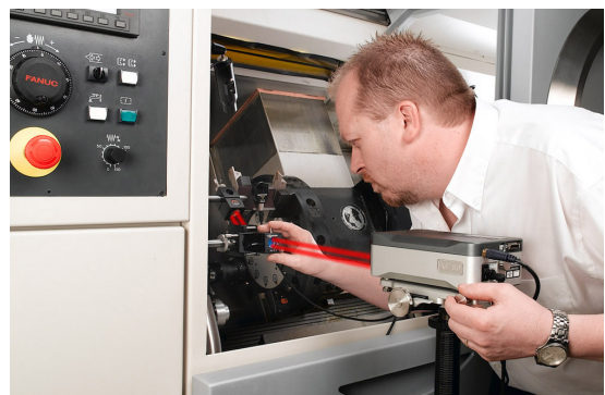
Calibrating a machine with a laser interferometer
