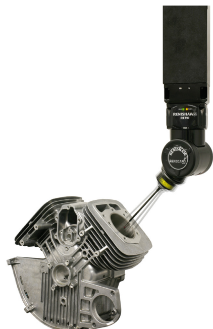
5-axis scanning technology is revolutionising CMM inspection
