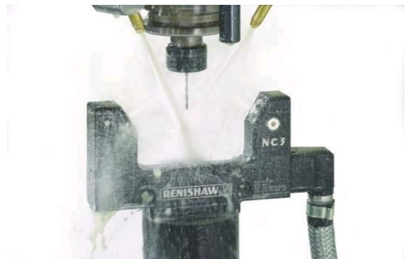
Figure 11 – checking broken tools with the coolant system still active
