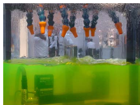
Figure 6 – demonstration of MicroHole™ protection with tool setter fully submerged
