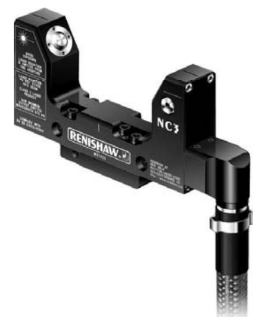
Figure 14 – Renishaw NC3 fixed system is typically mounted to the machine bed. Compact transmitter and receiver units allow for setting of tools up to 75 mm diameter in a footprint on just 135 mm x 26 mm
