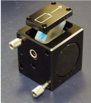
Photograph 5 - removal of the optics cartridge
