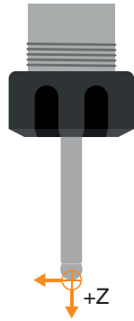
2 Manually set a nominal tool frame where +Z points out of the artefact
