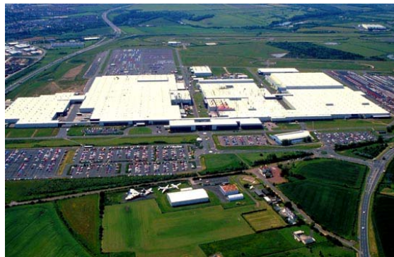
Nissan's Sunderland plant – main suppliers are grouped on the periphery of the site so all parts are made in-situ
