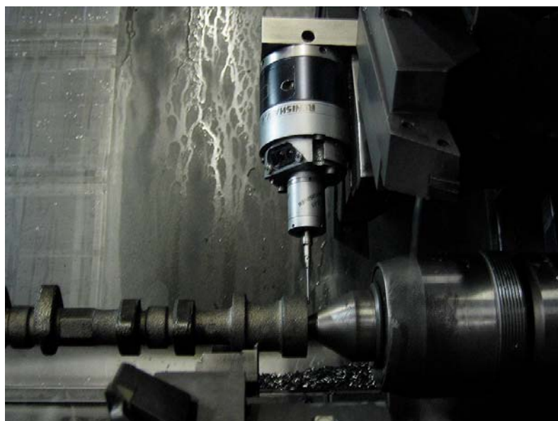
Renishaw LTO2S/LP2 probe system mounted on a twin turret CNC lathe – accurately locates the front face prior to machining, all in a cycle time of 90 seconds
