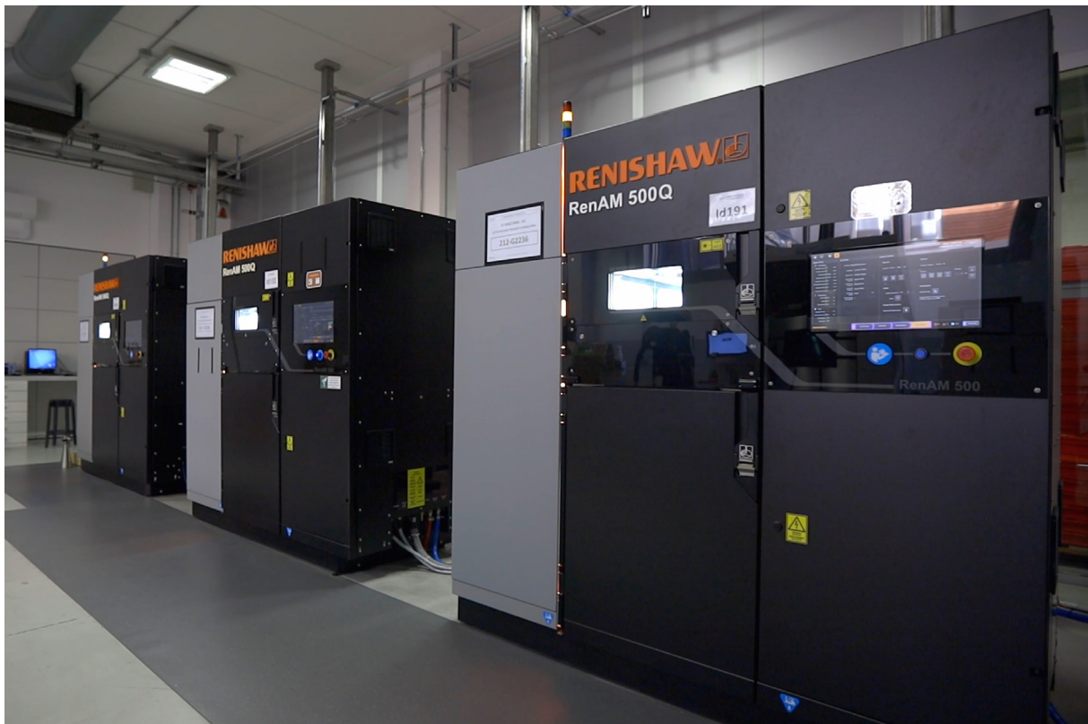
The RenAM 500Q system enables large volume production due to its four high-power 500W lasers
