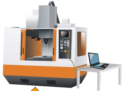
Using a data transfer cable
