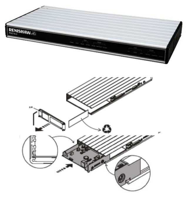
Fitting the PI 200-3 interface card to the PHC10-3
