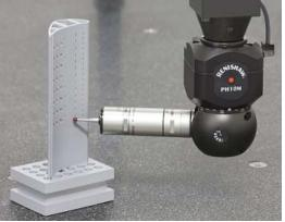
As a consequence of this work, Renishaw is pleased to announce the reduction of the repeatability specification of the PH10 from 0.5  $\mu$ m (2 $\sigma$ ) to 0.4  $\mu$ m (2 $\sigma$ ).
