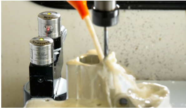
The Renishaw NC4 system is used to prevent damage caused by damaged tools to very expensive parts - eliminating resultant scrap, re-machining and wasted time.
