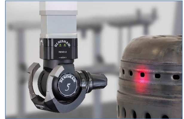
REVO Vision Probe (RVP) System - vision inspection system using REVO's infinite positioning and 5-axis motion capability. A solution for parts with large numbers of holes that can't be accurately measured with tactile probing or manual methods.
