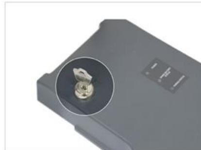
MCU W-2 locking position OFF, joystick deactivated
