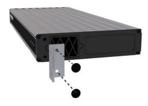
The rack mounting kit (Renishaw part number A-5518-0005) contains two brackets and four M5  $\times$  6 mm screws. Assemble the brackets to the UCC BI as shown below:
