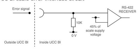
The UCC BI supports the error signal provided by Renishaw's digital incremental encoders. The UCC BI can also detect tri-state conditions on the A and B signals. If the error signal is not integrated into the connected encoder, then the user should connect pin 3 (Error - ) to pin 7 (+V scale).
