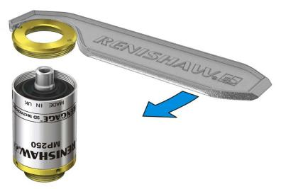
7. Remove the diaphragm positioning tool. Refit stylus and recalibrate probe (for more information, see **page 3-2**, "Fitting the stylus" and **page 3-6**, "Calibrating the MP250").
