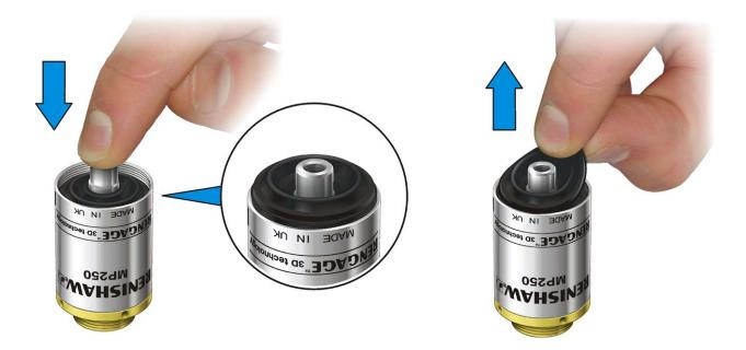
2. Screw the diaphragm positioning tool (Renishaw part no. A-5500-1652) supplied with the diaphragm replacement kit into the stylus holder.
