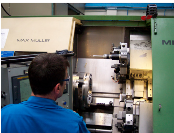
Turret probing and a removable tool setting arm on a machine that has been retrofitted with a Fanuc control, solely to integrate the probing systems
