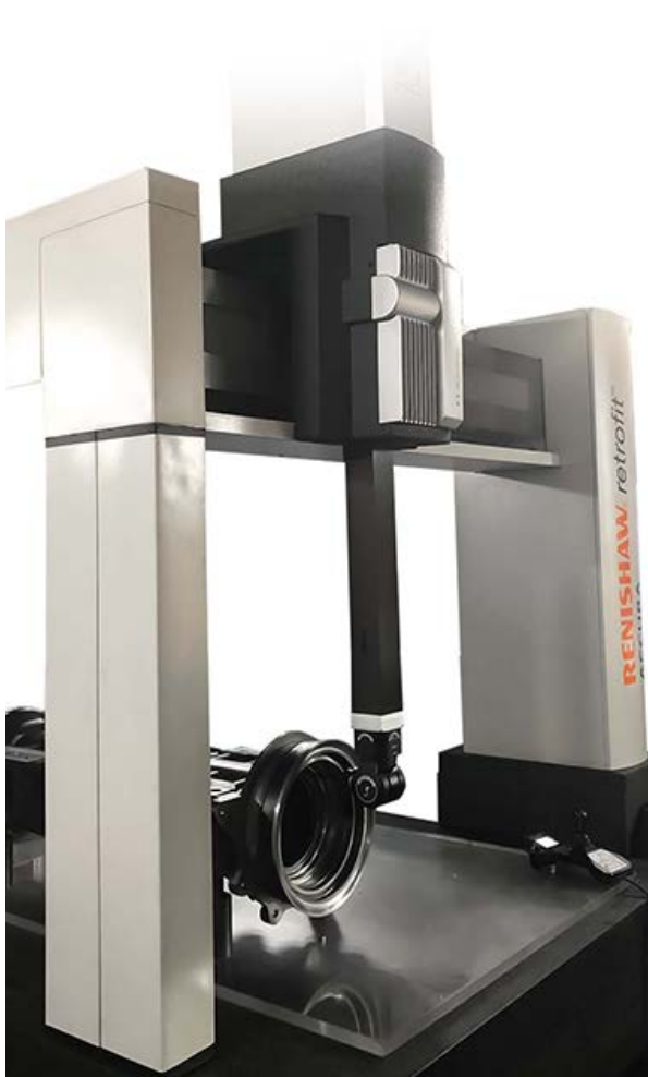
REVO measuring a cannon tube used in the locomotive industry
