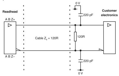
Standard RS422A line receiver circuitry. Capacitors recommended for improved noise immunity.
