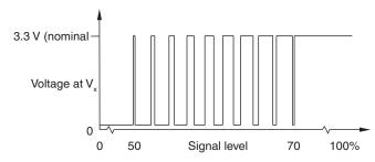
Between 50% and 70% signal level,  $\rm V_{\rm X}$  is a duty cycle. Time spent at 3.3 V increases with incremental signal level.
