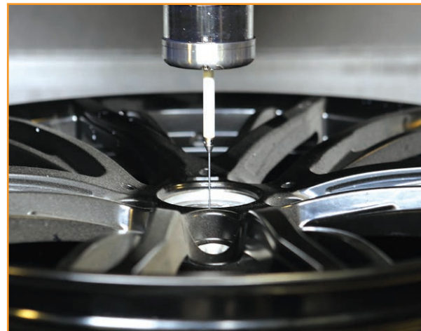
RMP60 measuring the alloy wheel mounting surface
