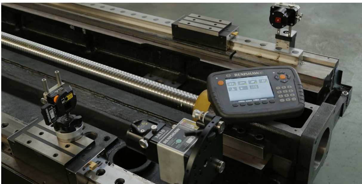
Using the XK10 to measure the parallelism of two guide rails
