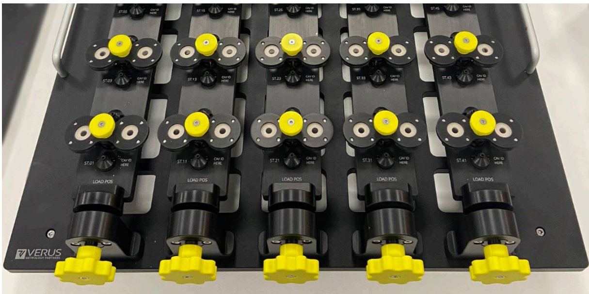
A bespoke Verus 48-station fixture for measuring soft rubber components
