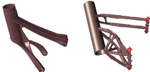
1. CAD model of seat post designed for aluminium alloy casting
