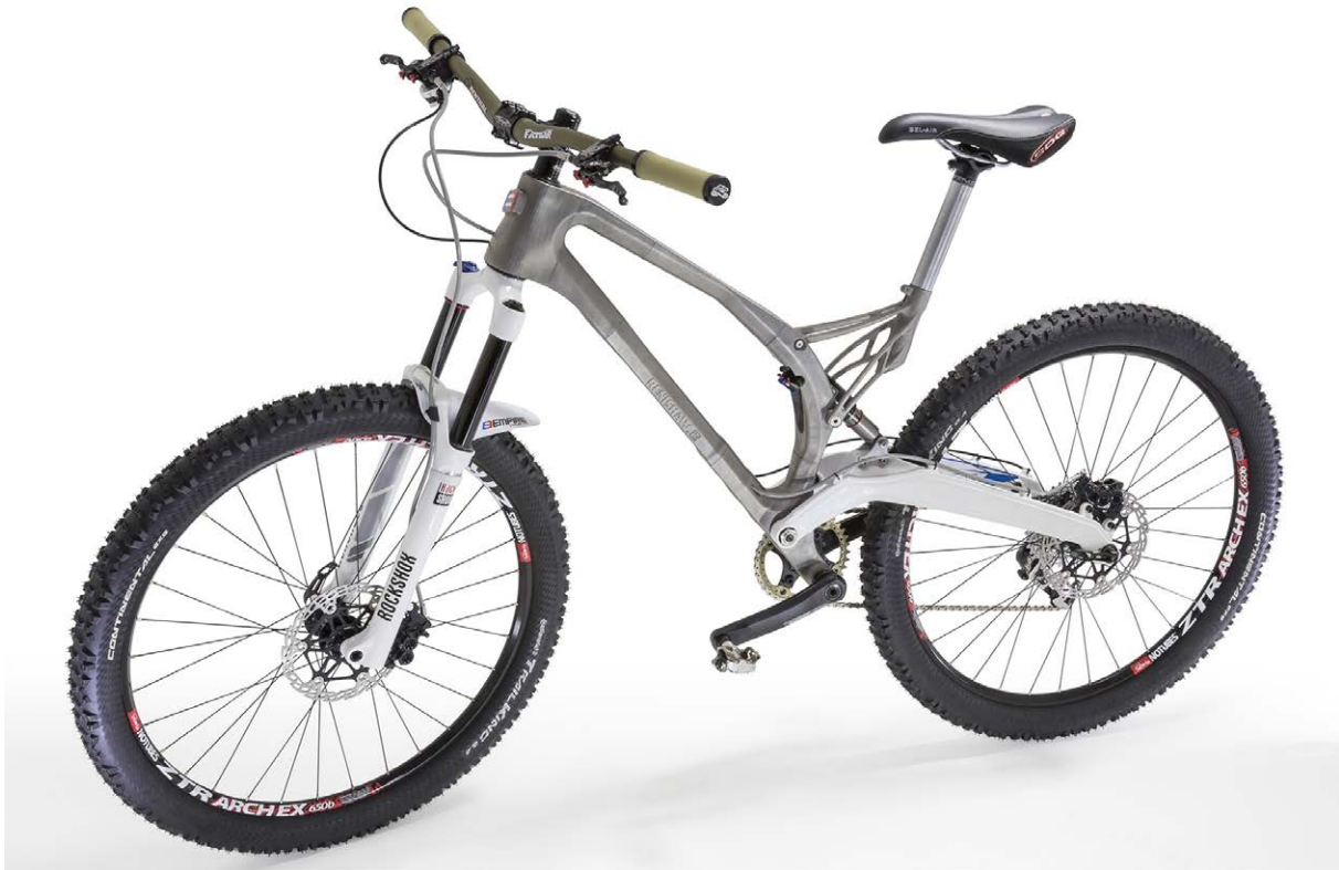
Complete bike with 3D printed titanium alloy frame and seat post bracket
