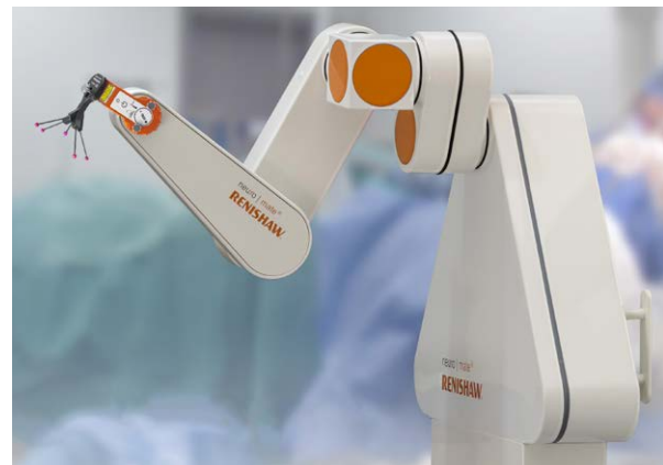
neuromate stereotactic robot with neurolocate frameless patient registration module
