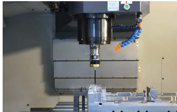
RMP600 probing the mould plate
