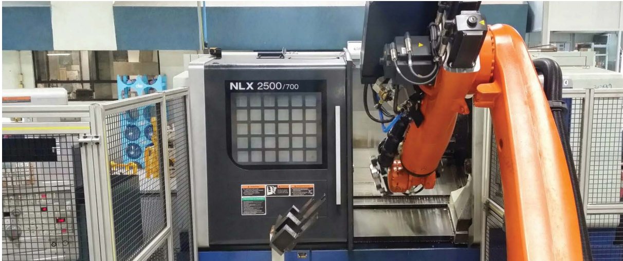
A work cell is formed by two lathes, a marker, a part device detector, the robot and the Equator gauging system.
