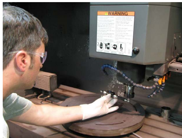
Getting hands-on with the wireless ballbar at Silfex
