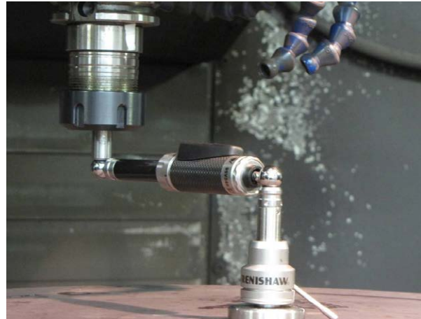
QC20-W wireless ballbar performing a test on a VMC
