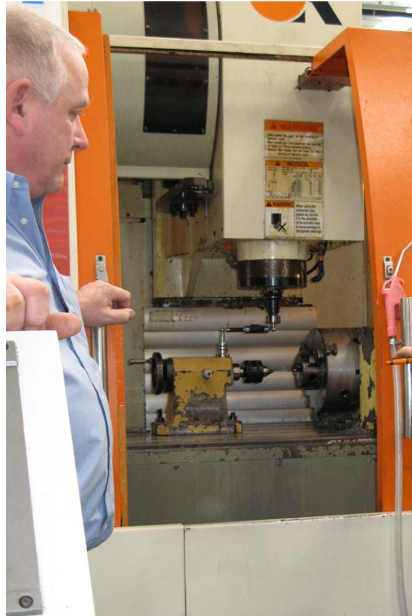
Bob Monkhouse carrying out a pre-qualification test using a Renishaw QC20-W ballbar
