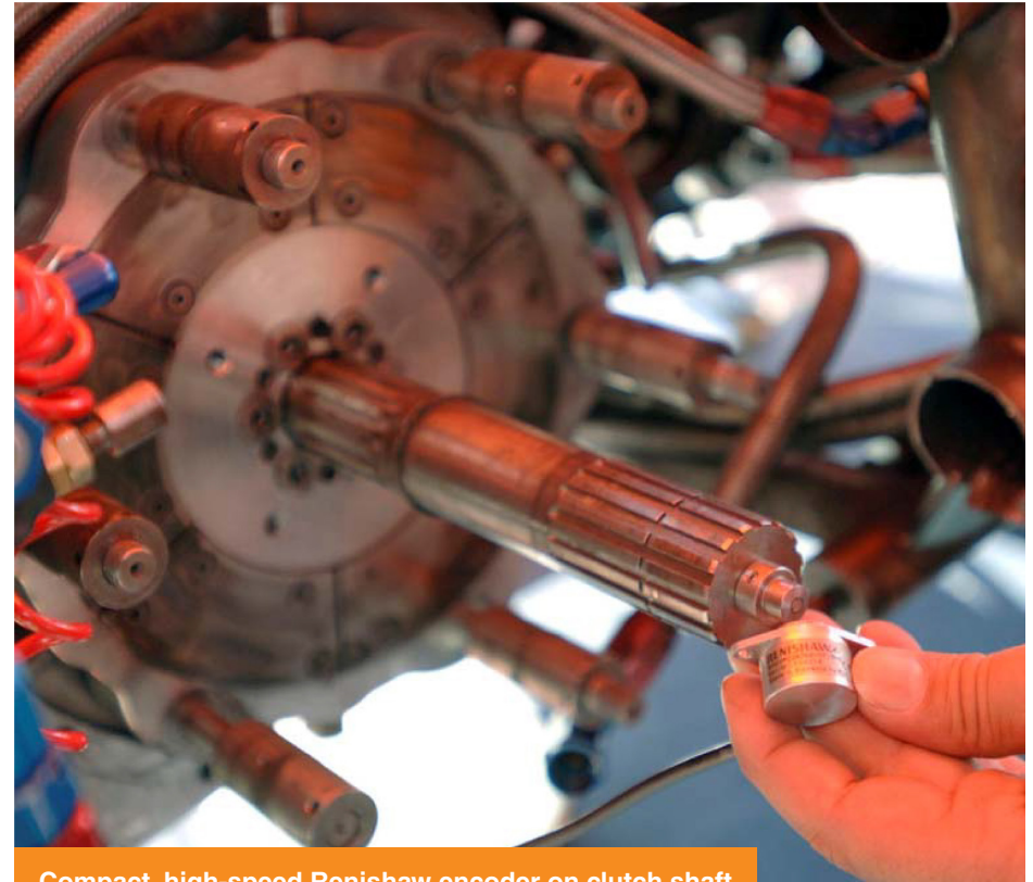
Compact, high-speed Renishaw encoder on clutch shaft
