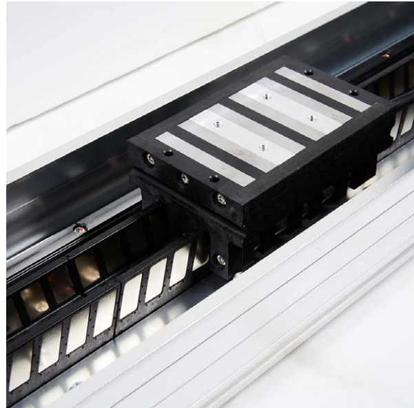
KOVERY linear motor with two permanent magnet tracks
