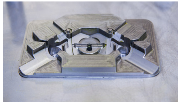
Complex mould tools are easily set up using the Renishaw touch-trigger part setting probe
