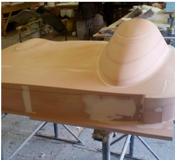
The 16 sections had to fit together accurately to ensure that the fibreglass mould would require the minimum of hand finishing
