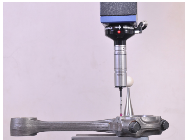
Con-rod master being 'calibrated' on a CMM in a temperature controlled room.
