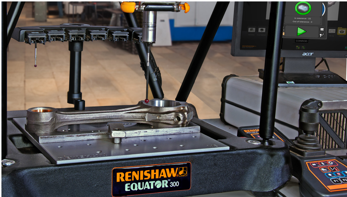
Kishan con-rod on fixture plate on Equator 300
