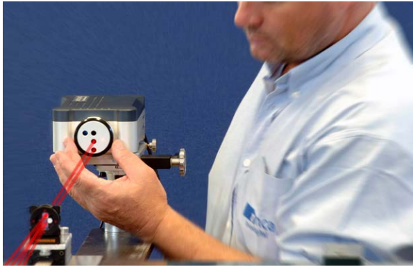
The Renishaw XL-80 calibrating a printer axis
