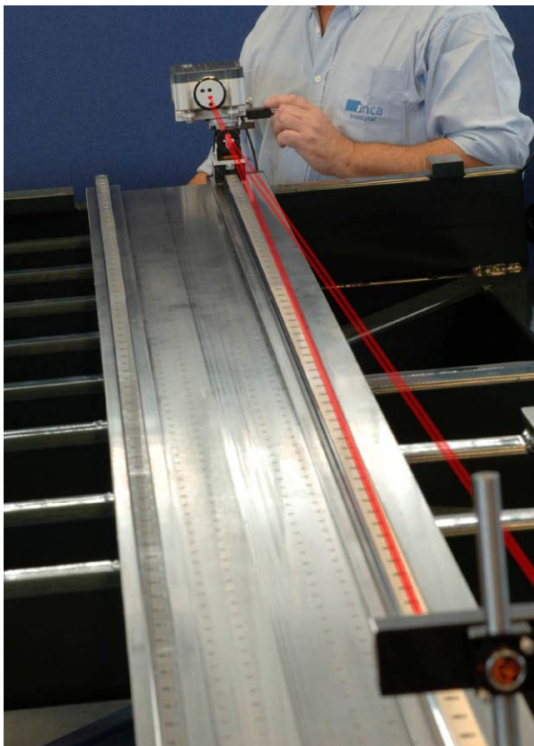
Machine guide rails can be up to 11.5 m - the XL-80 is more than capable of calibrating the full length of the table at the machine’s top speed
