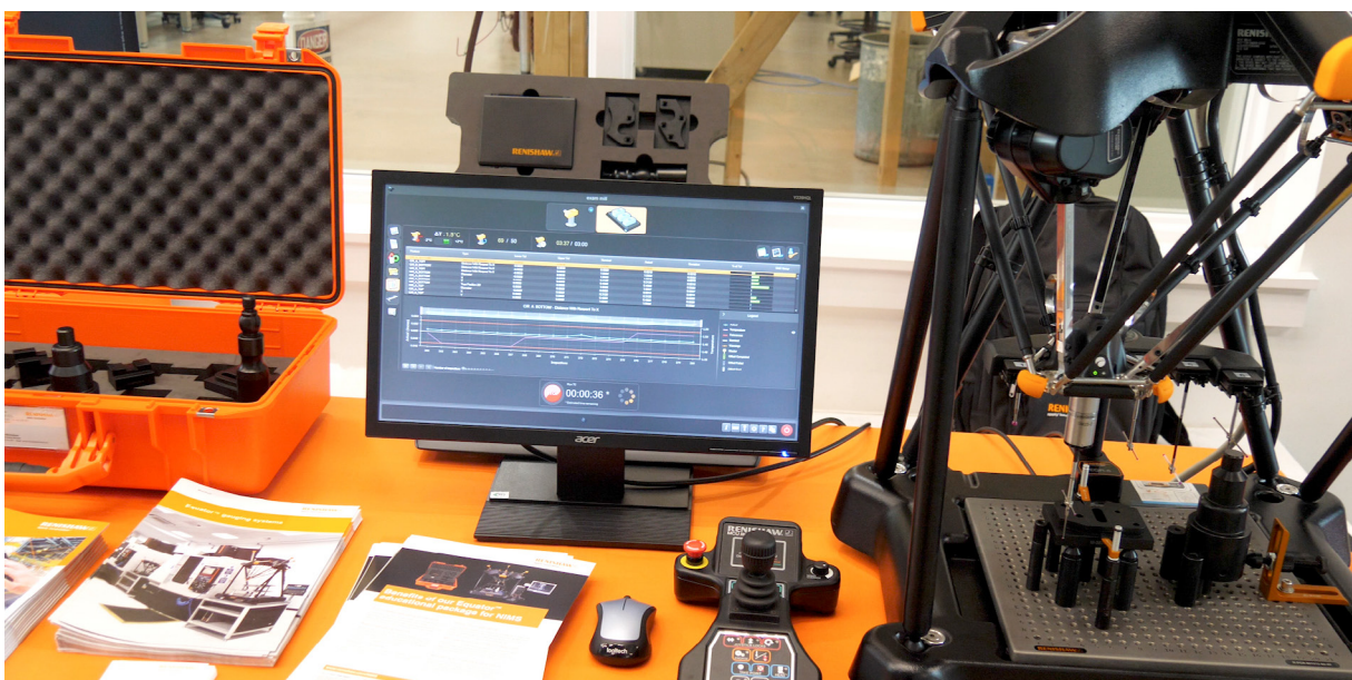
The Equator gauging package for NIMS includes prewritten programmes, styli, two metrology fixturing plates, and fixturing that fits all 13 parts
