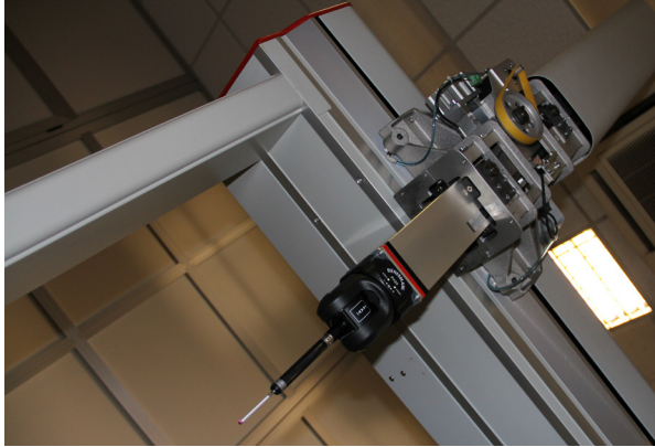
PH20 probe head mounted on COORD-3 CMMs for 5-axis measurement
