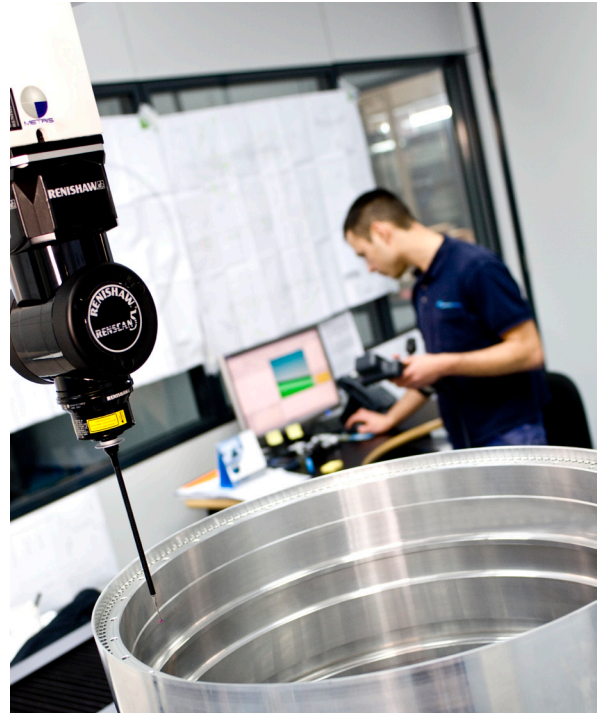
REVO® scanning a large bore on an aerospace component.
