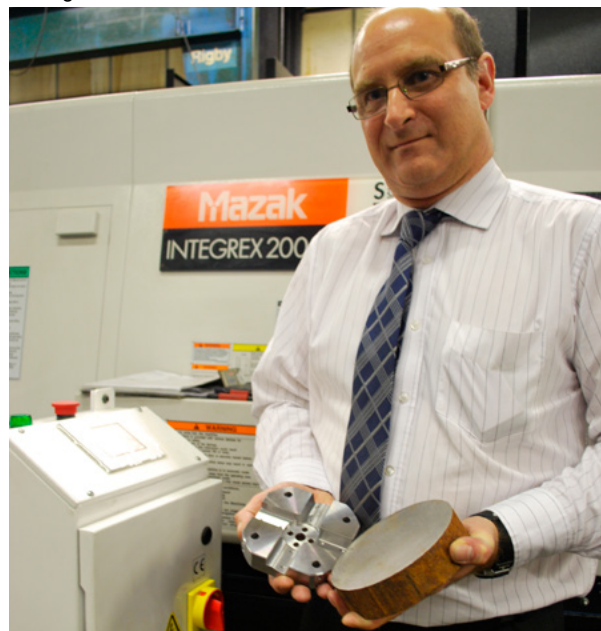
Steve Randerson with billet and finished part produced on the Mazak Integrex
