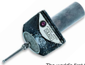
The world's first touch-trigger probe
