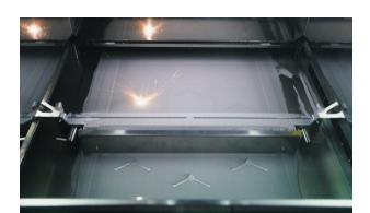
Traditional powder bed systems require the powder recoater to fully distribute powder before the layer can be consolidated. With TEMPUS technology, the lasers can fire at the same time as the recoater is moving.
