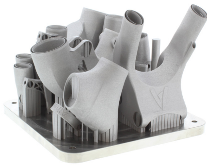
Atherton bike lugs on a build plate
