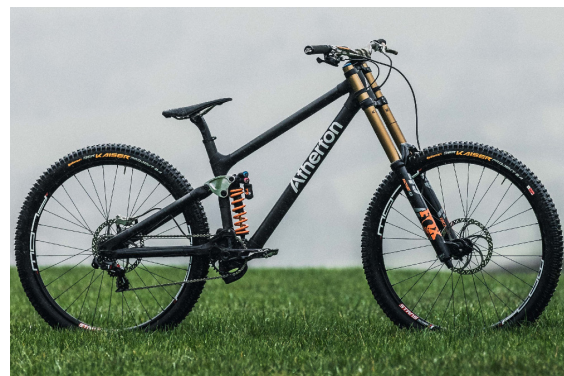
The Atherton Bikes design uses titanium nodes connected by carbon fibre tubes, combining the best of these two high-performance materials.
