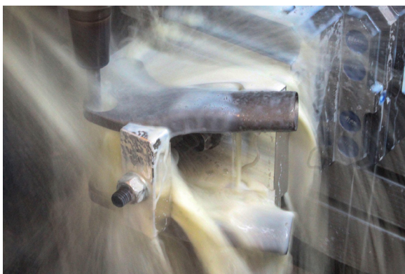
Machining of the 'yoke' - a key component of the rear suspension. Cutting of the precision bearing holes is performed on a 5-axis machining centre, using probing to establish datums and control tool wear to meet the required tolerances.
