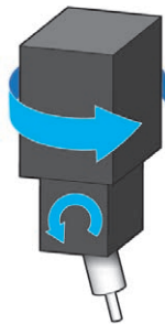
ISO 10791-6 reference = ' AK ' Head - Head machines 2 rotary axes in the spindle head
