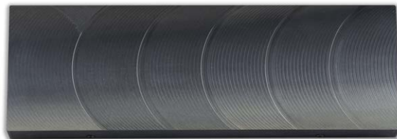
Figure 4: Test piece with six cuts representing six different levels of surface condition
