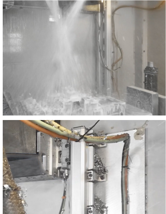
Figure 3. Using air purge on encoders stops contamination entering the encoder enclosure, even in extreme conditions.
