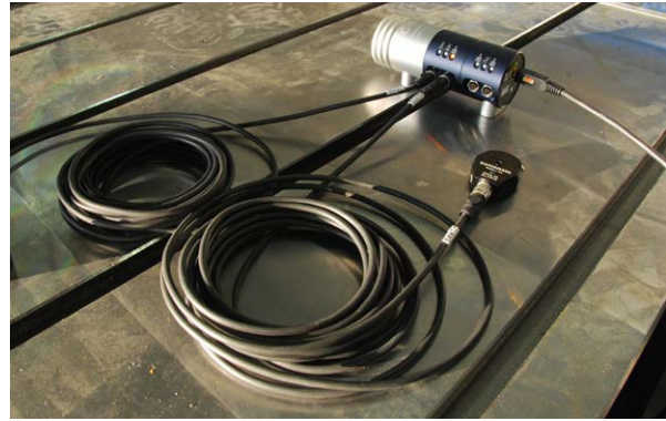
Sensors connected to the XC-80 compensation unit measure temperature and air pressure, allowing tests in any conditions
