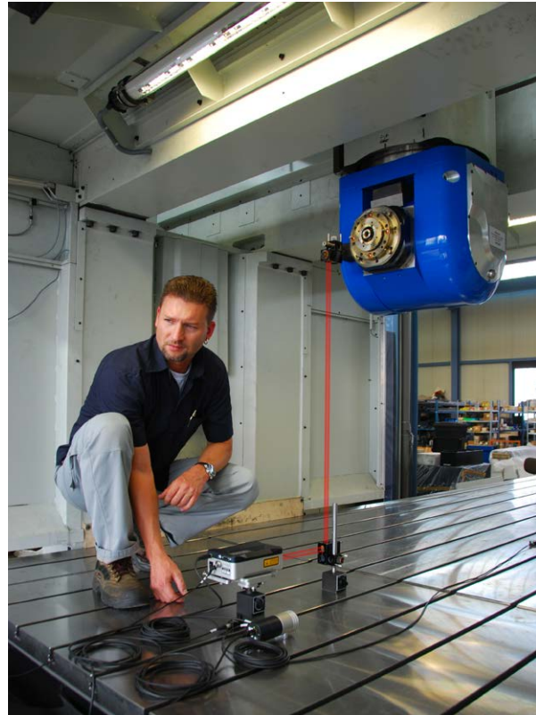
Jürgen Emslander can test accuracy with the compact XL-80 in many more positions, even inside machines like this Edel
