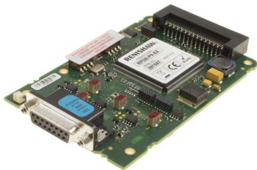
RPI20 parallel interface - interpolates 158 nm sine / cosine signals to produce parallel output with LSB resolutions of 77.2 picometres (38.6 picometres available)
