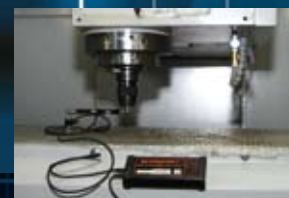
Quaser use a Renishaw QC10 to perform tests to 'double-ballbar' standard.
