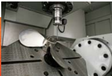
Above and right: RMP600 high-accuracy touch probe.
