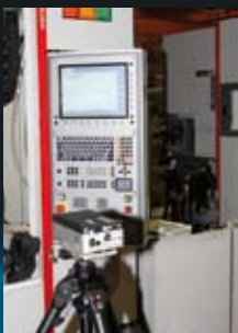
XL-80 being used to check for machine performance accuracy.
