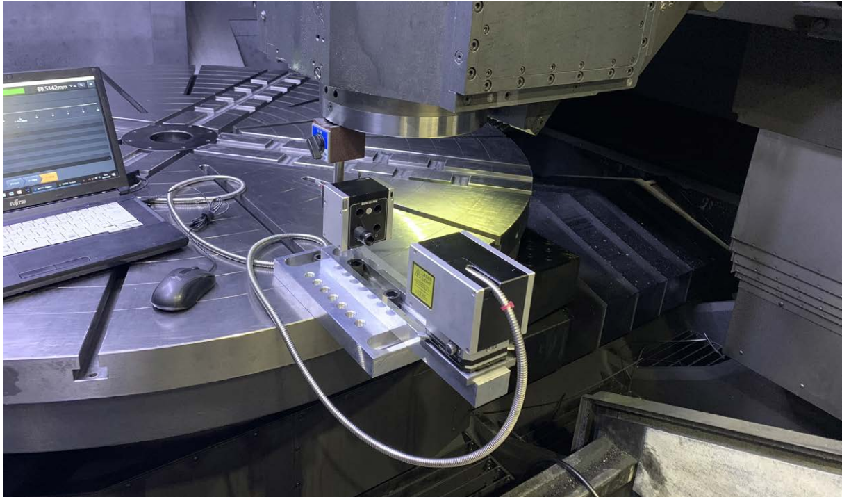
Measuring machine tool accuracy with the XM-60 multi-axis calibrator
