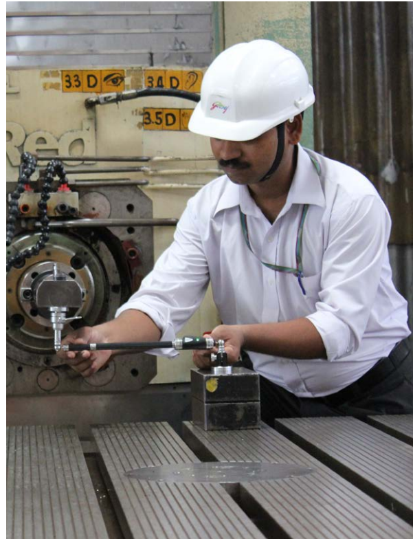
QC20-W ballbar test set-up in Godrej manufacturing facility
