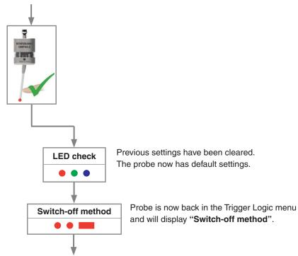
3. Configure probe settings as required using Trigger Logic.
